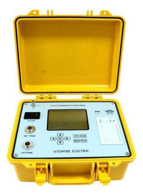
Weshine® Turns Ratio Tester for testing Transformer Voltage Ratio
